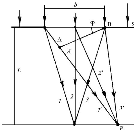
FIG. 1. Scheme of the Fraunhofer diffraction by the slit.
