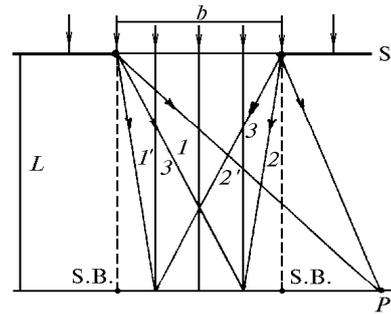
FIG. 2. Scheme of diffraction of the edge and directly transmitted rays for Fresnel's diffraction by the slit.
