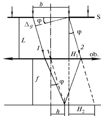
FIG. 3. Scheme of formation of Fraunhofer's diffraction pattern from a slit in the objective focal plane.
