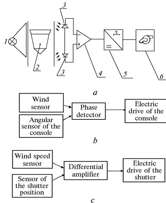
FIG. 2. Block-diagram of the air flow regulator (a), block-diagrams of the sampling console (b) and shutter (c) control.
