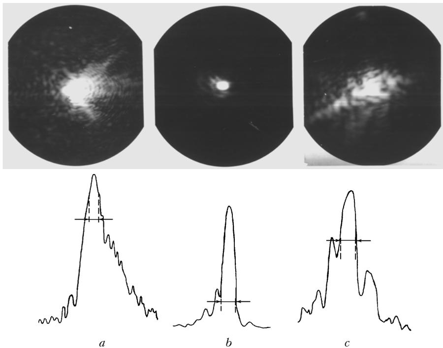
FIG. 4. The photographs of the focal spots and the densitograms of the radiation, reflected from the nonlinear medium and passed again through the optical channel. The diameter of the extended beam is equal to 150 mm, (a) and 75 mm, (b, c). The wave front on the last photographs was distorted additionally by the heating of the area of the optical channel.
