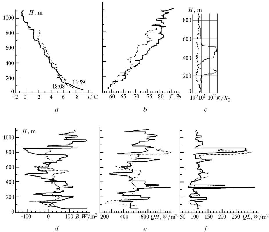
FIG. 3. Vertical profiles of temperature (a), humidity (b), scattering coefficient (c), radiation budget (d), down going radiation (e), and up going radiation (f) on September 29, 1996 over Tomsk: solid lines – ascent of the deltaplane; points – descent.
