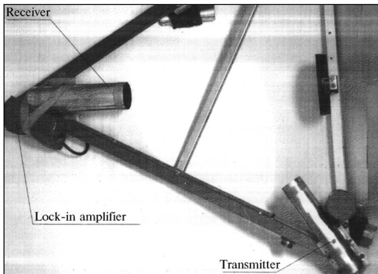
FIG. 2. External view of the nephelometer.
