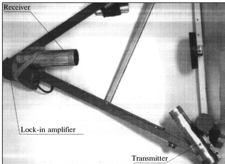
FIG. 2. External view of the nephelometer.
