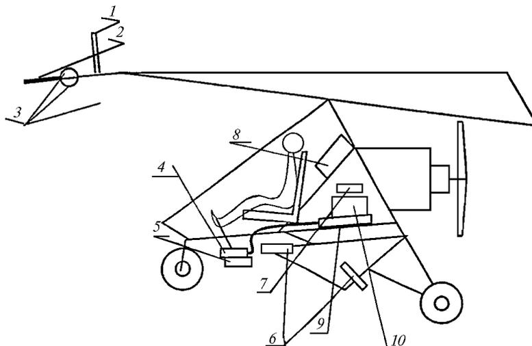
FIG. 1. Arrangement of scientific instrumentation on the deltaplane: 1) cloud irradiance sensor, 2) radiation budget meter, 3) pyranometers, 4) the block of sensors of air temperature and humidity, 5) filter setup, 6) nephelometer, 7) pressure sensor, 8) onboard recording complex, 9) air flow stimulator, and 10) battery.
