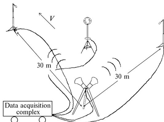
FIG. 1. Block-diagram of the experiment.
