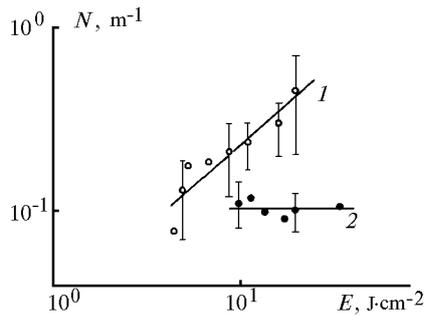
FIG. 2. Dependence of the linear concentration of optical break down cells on the laser radiation energy density: (1) 15 min fog lifetime on the measurement path, (2) 30 min and longer lifetime.
