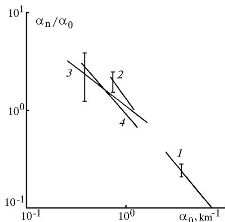
FIG. 3. Influence of the atmospheric optical and meteorological state on the nonlinear extinction coefficient for  $\text{CO}_2$  laser radiation: (1) fog, (2) drizzle, (3) rain, and (4) snow.
