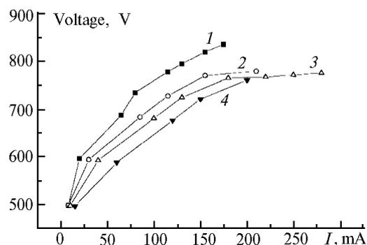
FIG. 1. Volt-ampere characteristics of the discharge obtained at different repetition frequencies of the preionization pulses,  $f$ ; at  $f = 10$  kHz (curve 1); 15 kHz (curve 2); 20 kHz (curve 3) and 30 kHz (curve 4).
