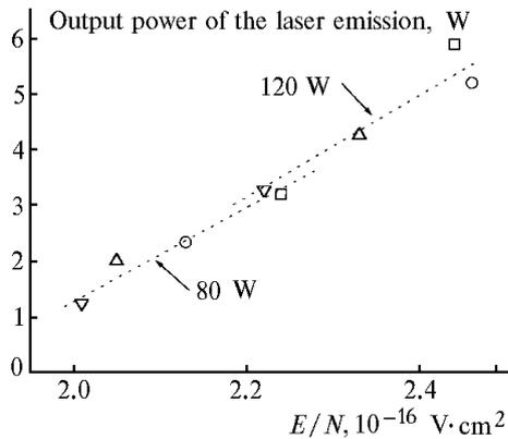
FIG. 3. The output power of the laser emission as a function of the reduced strength of the electric field.  $f = 10$  ( $\square$ ),  $15$  ( $\circ$ ),  $20$  ( $\Delta$ ), and  $30$  kHz ( $\nabla$ ).
