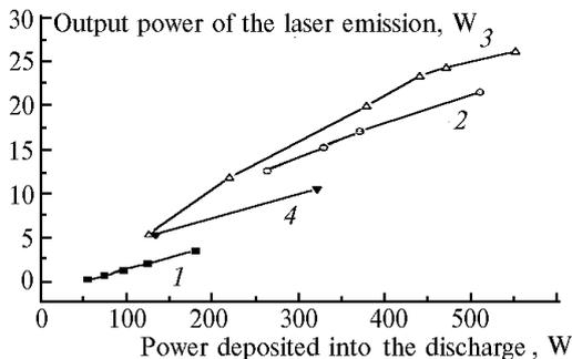
FIG. 4. The output power of the laser emission as a function of the electric power deposited into the discharge at different pressures of the gas mixture.
