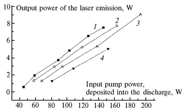
FIG. 2. The output power of the laser emission as a function of pump power deposited into the discharge. Preionization conditions are the same as those shown in Fig. 1.
