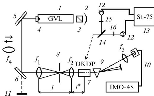
FIG. 1. The optical arrangement of the experiment: CVL (1), resonator mirrors (2, 4), Glan prism (3), beam folding mirrors (5, 6), input ( $f_1$ ) and output ( $f_2$ ) lenses of the collimator, crystal (7), diaphragm (8), quartz prism (9), CaF<sub>2</sub> lens ( $f_3$ ), power meter (10), screen (11), lens ( $f_4$ ), photocells (12), oscilloscope (13), beam splitter (14), and optical filters (15, 16).
