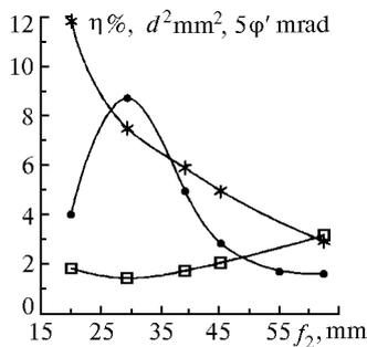
FIG. 3. Dependence of SFG efficiency and beam parameters on the focal length of the collimator output lens  $f_2$ : efficiency  $\eta$  (●—●);  $\varphi'$  (\*—\*); the squared diameter  $d^2$  (□—□).
