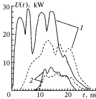
FIG. 2. The pulses  $U(t)$  of the CVL radiation power:  $\varphi = 7.7$  rad (1),  $\varphi = 0.2$  rad (2),  $\lambda = 0.51 \mu\text{m}$  (solid curve),  $\lambda = 0.578 \mu\text{m}$  (dashed curve).
