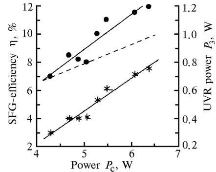
FIG. 4. SFG efficiency and UVR power as functions of the incident power  $P_c$ : UVR power  $P_3$  (\*—\*), efficiency  $\eta$  (●—●), theoretical calculation of  $\eta$  (dashed line).
