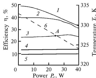
FIG. 5. The efficiency  $\eta(\phi', P_c)$  calculated as a function of  $P_c$  at  $I_1 = I_2 = 0.65 \cdot 10^5$  W/cm<sup>2</sup>: Curves 1, 2, 3, 4, and 5 correspond to  $\phi' = 0.2, 0.35, 0.7, 1.4, 2.1$  mrad, respectively; 6 corresponds to temperature,  $T_c$ , at a crystal side.
