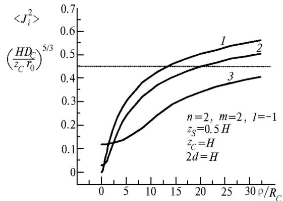
FIG. 5. Distribution of the error over the object when using the modified correction method at different size of the averaging zone.  $R_0 = 0$  (1) (correction using the central point),  $R_0 = 2R_C$  (2), and  $R_0 = 10R_C$  (3).
