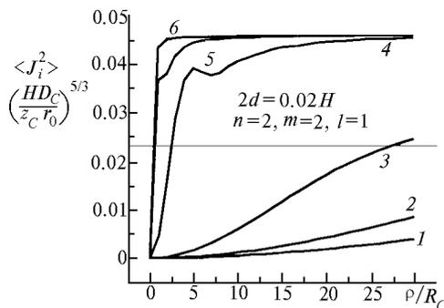
FIG. 3. Residual error as a function of the distance from a point on the object to its center. The corrector is positioned at the layer image center (1-3) and in the receiving aperture plane (4-6):  $z_S = z_C = 0.8H$  (1);  $z_S = z_C = 0.5H$  (2);  $z_S = z_C = 0.2H$  (3);  $z_S = 0.8H, z_C = H$  (4);  $z_S = 0.5H, z_C = H$  (5);  $z_S = 0.2H, z_C = H$  (6).
