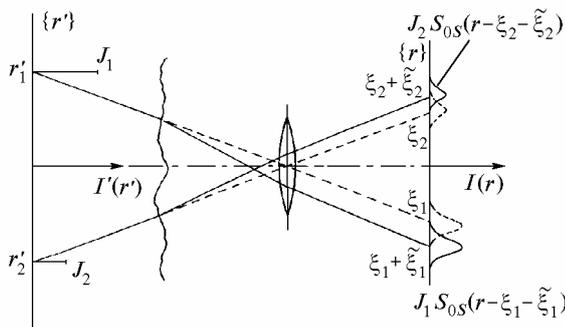
FIG. 2. The scheme of constructing the algorithm of  $\tilde{I}(\mathbf{r})$  realization for a short-exposure image in the case with a two-point object;  $\mathbf{r}'_1, \mathbf{r}'_2$  are the coordinates of points in the object plane;  $J_1, J_2$  are their radiation powers;  $\xi_1, \xi_2$  are the geometrical-optical displacements of points in the image plane.
