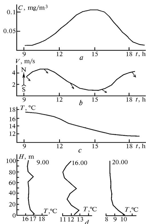
FIG. 1. Diurnal dependence:  $\text{SO}_2$  concentration (a), wind direction and velocity (b), air temperature (c), vertical temperature distribution in the 100-m layer (d).
