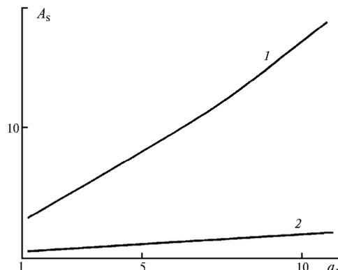
FIG. 4. Relation of the asymmetry parameter  $A_s$  and the asymmetry factor of the scattering phase function of an elementary volume for  $\Lambda = 1$ :  $\tau = 1$  (curve 1) and  $\tau = 10$  (curve 2).
