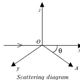
We assume that light is incident along the positive  $x$  direction. The viewing direction  $OA$  is in the plane  $XY$  and makes the angle  $\theta$  with the incidence direction of the beam. Integral parameters are being determined depending on which viewing direction is chosen. Thus, for instance, for the direction along the  $X$  axis
