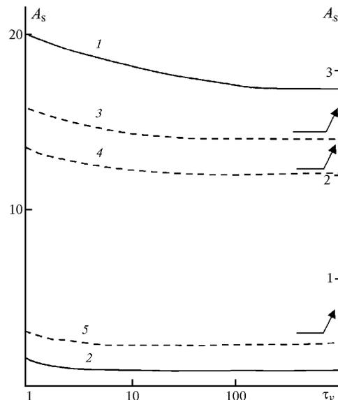
FIG. 3. Dependence of the asymmetry parameter  $A_s$  on the transverse optical depth  $\tau_y$  of the medium for  $\Lambda = 1$ :  $\tau_x = 1$ ,  $\tau_z = 1$ , and  $a_{x2} = 12.09$  (curve 1);  $\tau_x = 10$ ,  $\tau_z = 1$ , and  $a_{x2} = 12.09$  (curve 2);  $\tau_x = 1$ ,  $\tau_z = 1$ , and  $a_{x1} = 1$  (curve 3);  $\tau_x = 10$ ,  $\tau_z = 10$ , and  $a_{x1} = 1$  (curve 4); and  $\tau_x = 10$ ,  $\tau_z = 1$ , and  $a_{x1} = 1$  (curve 5).
