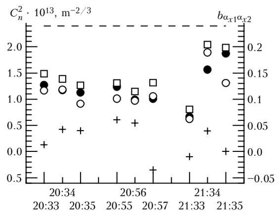
FIG. 2. Comparison of  $C_n^2$  values measured by the single-channel scheme and by the differential technique: differential scheme ( $\square$ ); simultaneous measurements by meters I and II ( $\bullet$ ,  $\circ$ ); coefficients of cross correlation between the signals from the I and II meters of the angular displacements of the image ( $+$  - ); the calculated value is shown by the dashed line. Realization length is 40 seconds. The distance between the sub-apertures on the X axis is 68 mm.
