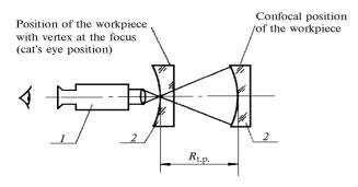
FIG. 1. Geometry of the autocollimation technique to measure the curvature radius: an instrument controlling adjustments (1); a test piece (2).
