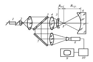
FIG. 2. Optical arrangement of the interferometer by the Fizeau scheme: laser (1), widener of a laser beam (2), beamsplitter (3), illuminating objective lens (4), aplanatic meniscus (5), test piece (6), beam-turning mirror (7), TV camera (8), video controller (9), interferogram processing device (10); F'is the interferometer focus.
