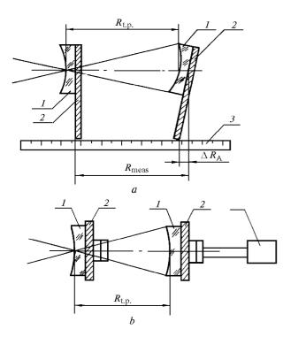
FIG. 3. The radius measurement error  $\Delta R_A$  due to violation of the Abbe principle: test piece (1); test piece holder mounted through a bracket to a meter (2); meter with the measurement scale (3); laser meter of displacements (4).
