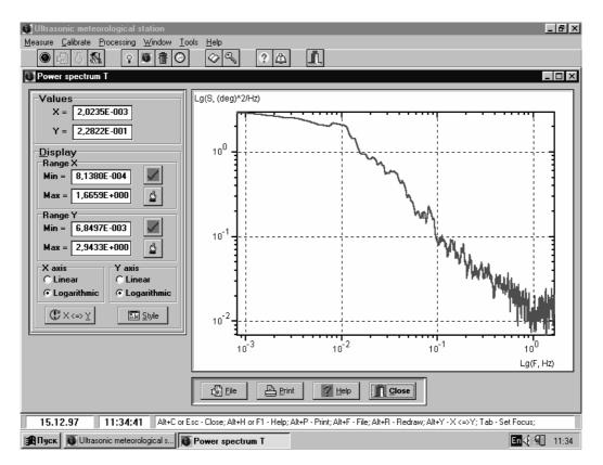
FIG. 4. METEO 2.0 Windows Application: the window for graphical data obtained at secondary processing of the measured results (the window displays the power spectrum of turbulent fluctuations of air temperature).
