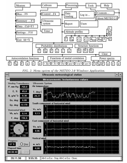
FIG. 3. METEO 2.0 Windows Application: the window for current measured data.
