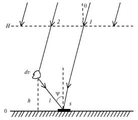
${\bf Fig.}~{\bf 2.}$  The scheme for calculation of incoming solar radiation fluxes.
