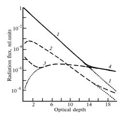
Fig. 1. The dependence of the fluxes of direct (1), single scattered (2), and multiple scattered (3) radiation on the optical depth.
