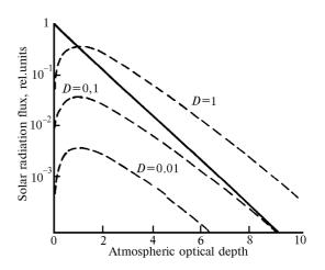
Fig. 3. The dependence of solar radiation fluxes on the slant optical depth of the atmosphere.
