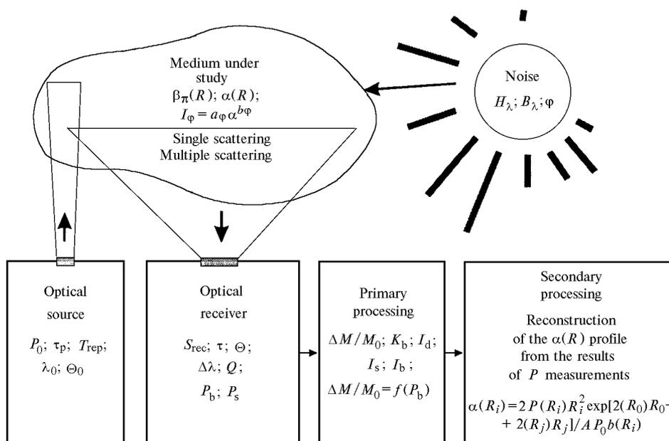
Fig. 1. Model of a lidar system.
