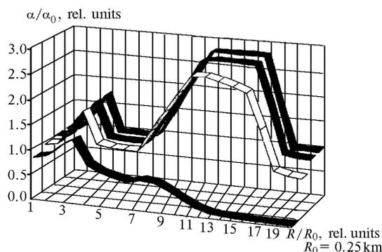
Fig. 4. Reconstruction of the scaled volume extinction coefficient  $\alpha/\alpha_0$  by the method of successive layers in the absence of the background under different atmospheric conditions; from the top down: model profile;  $\alpha_0 = 0.03 \text{ km}^{-1}$  (clear sky);  $\alpha_0 = 0.1 \text{ km}^{-1}$  (a light haze);  $\alpha_0 = 1.0 \text{ km}^{-1}$  (a moderate haze).
