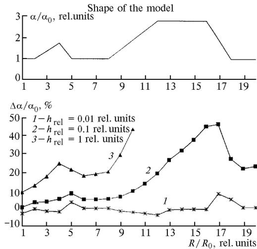
**Fig. 5.** Relative error of reconstruction of the volume extinction coefficient  $\alpha$  by the method of successive layers with compensation for the background by the traditional method under different background conditions for  $\alpha_0 = 0.03 \text{ km}^{-1}$ ;  $R_0 = 0.25 \text{ km}$ .
