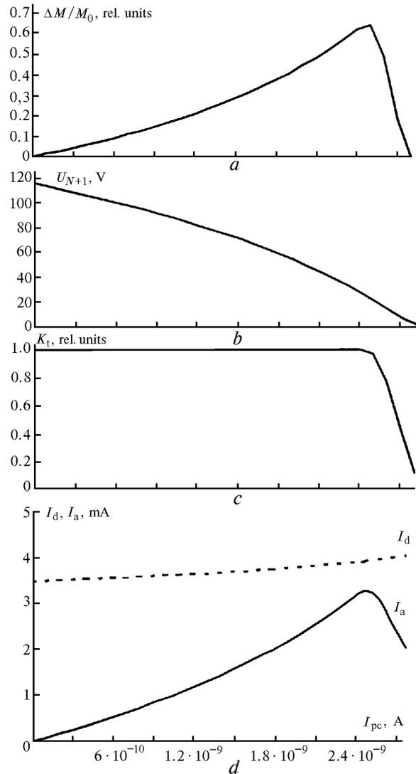
**Fig. 3.** Change of the PMT characteristics: relative gain coefficient  $\Delta M/M_0$  (a); the voltage at last dynode-anode gap (b); transmission coefficient of the last PMT stage (c); current through the voltage divider and the background anode current (d) vs. the background current of the photocathode  $I_{pc}$ .
