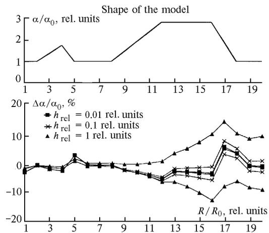
**Fig. 6.** Relative error of reconstruction of the volume extinction coefficient  $\alpha$  by the method of successive layers based on compensation for the background with the allowance for the noise of the photodetector under different background conditions at  $\alpha_0 = 0.03 \text{ km}^{-1}$ ;  $R_0 = 0.25 \text{ km}$ .
