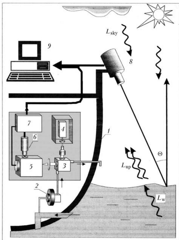
**Fig. 2.** The scheme of drawing-through the water and measurements of the fluorescence spectrum of the seawater: ship body (1); pump for water intake and drawing through the plastic pipe line (2); cell (3); the laser (4); scanning monochromator (5); photomultiplier tube (6); the ADC and monochromator control unit (7); a POLAS spectrometer (8); a computer (9).
