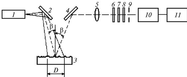
**Fig. 1.** Block-diagram of the model set-up: laser (1); plane mirrors (2 and 4); piece of asphalt cover (3); lens (5); interference filter, neutral density filter, and a polarization analyzer (6, 7, and 8); aperture diaphragm (9); photodetector (10); digital voltmeter (11).
