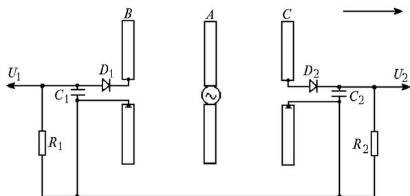
**Fig. 3.** Block-diagram of the recording technique of the dielectric constant variation at the line separating two media. *A* is the transmitting antenna, *B* and *C* denote the receiving antennas.
