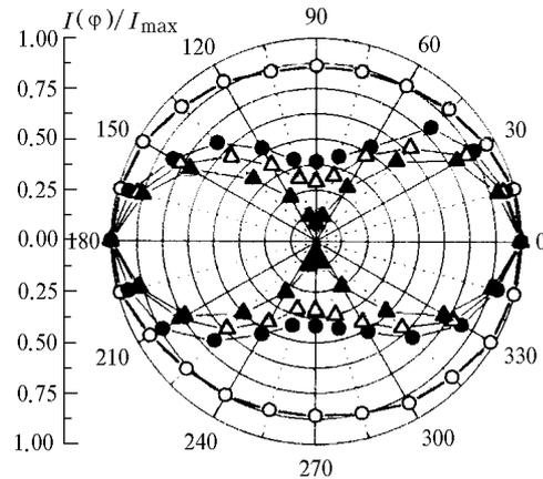
**Fig. 2.** Angular diagram of polarization degree of radiation reflected from the asphalt cover surface under different conditions of the surface: dry asphalt cover ( $\circ$ ); snow ( $\bullet$ ); wet asphalt cover ( $\Delta$ ); the ice cover ( $\square$ ).
