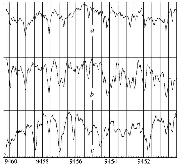
**Fig. 2.** CO<sub>2</sub> absorption spectrum in 1 μm region recorded at temperatures of 300 K (a), 1300 K (b), and in the electric discharge (c).
