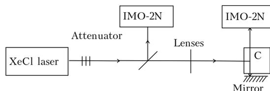
Fig. 1. Optical arrangement of the experimental setup; C denotes the cell with a solution.
