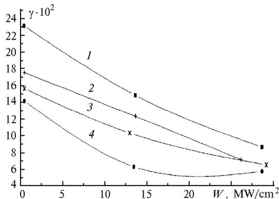
Fig. 2. Quantum yield of the photodecay vs. intensity of XeCl laser radiation: F-(2M)F (1), *trans*-stilbene (2), F-(3M)F (3), and F-(4M)F (4).
