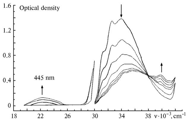
Fig. 3. Change of absorption spectrum of ethanol solution of *trans*-stilbene under exposure to XeCl laser radiation.
