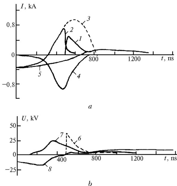
**Fig. 3.** Oscillograms of current and voltage at the setup operation with the load  $R_L = 58\ \Omega$  ( $C_1 = 4.4\ \text{nF}$ ,  $C_2 = 0$ ):  $I_1$  (1),  $I_2$  (2),  $I_2$  at the short-circuit opening switch (3),  $I_3$  (4),  $I_4$  (5),  $U_1$  (6),  $U_3$  (7), and  $U_2$  (8).
