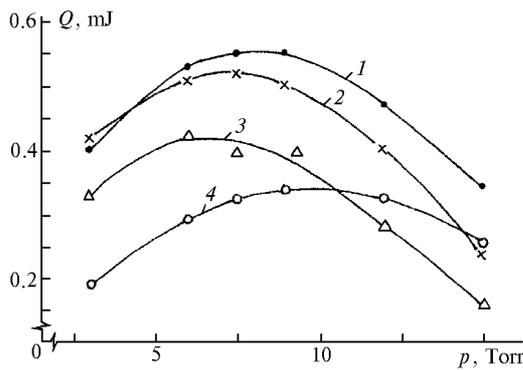
**Fig. 8.** Output energy of nitrogen laser vs. nitrogen pressure at 400 mm long discharge tube:  $d = 6.8$  mm,  $C_2 = 170$  (1), 330 pF (2), 0 (4) and  $d = 9.5$  mm,  $C_2 = 330$  pF (3).
