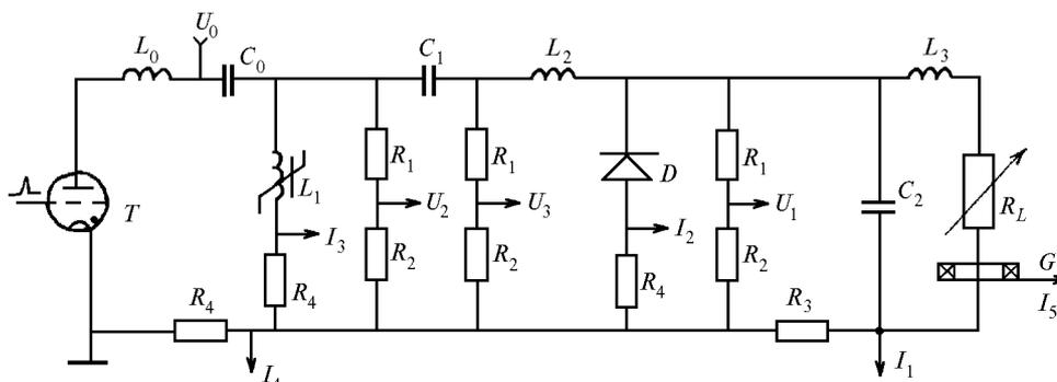
Fig. 1. Principal circuitry of the experimental setup with a semiconductor opening switch.
