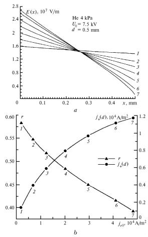
**Fig. 2.** Distribution of the electric field strength over the electrode gap length in a semi-self-maintained discharge (*a*), the value of the coefficient  $j_+(d)/j_+(0)$ , and the values required for the discharge maintenance the ion current density at the anode (*b*) calculated for some values of  $j_{e\,0}$ . Helium pressure equals 4 kPa,  $U_0 = 7.5$  kV, d = 0.5 mm.
