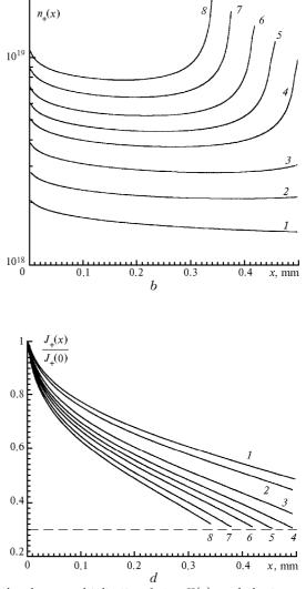
Fig. 1. Distribution of electric field intensity (a), ion density (b), the charge multiplication factor K(c), and the ion current density (d) over the interelectrode gap length at separate values of  $j_{e\,0}$ .
