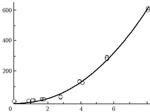
**Fig. 4.** Dependence of the energy of femtosecond Ti:Sa laser pulse absorbed by air on the laser pulse energy ( $a$ ,  $b$ ,  $c$  are fitting parameters;  $R^2$  is the correlation coefficient).
