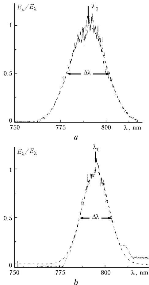
**Fig. 1.** Spectra of Ti:Sa laser pulses with  $\tau_p = 9 \text{ ns}$  (a) and  $80 \text{ fs}$  (b): dashed curves are for the results of fitting by the Gauss function;  $\lambda_0 = 790 \text{ nm}$  and  $\Delta\lambda = 23.4 \text{ nm}$  (a);  $\lambda_0 = 794.7 \text{ nm}$ ,  $\Delta\lambda = 17.7 \text{ nm}$  (b).
