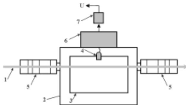
**Fig. 2.** PA detector: laser beam 1, body of the PA cell 2, concentrator 3, microphone 4, buffer volume 5, preamplifier 6, and filter 7.
