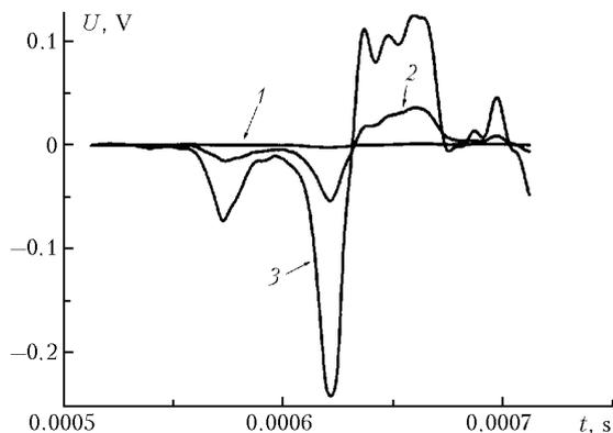
**Fig. 3.** PA signals generated at absorption of Ti:Sa laser pulses by indoor air.
