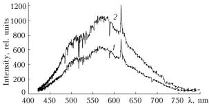
Fig. 4. The transmission spectra, for sunlight, of the film with 2% m/m FE luminophore additive: a fresh film [August 4 of 2002] (2), identical film after one-year storage [May 4 of 2003] (1). The spectra are not corrected for the spectral sensitivity of the photodetector used.
