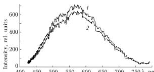
400 450 500 550 600 650 700 750  $\lambda$ , nm **Fig. 1.** The spectra of solar radiation before (1) and after (2) transmission through the film with the 0.1% m/m PE luminophore content. The spectra are not corrected for the spectral sensitivity of the photodetector used.
