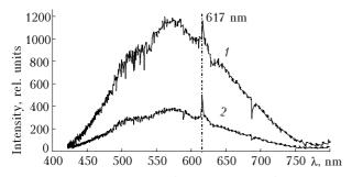
**Fig. 2.** The spectra of solar radiation transmitted through the HPPE film with 5% m/m addition of PLE luminophore (1) and transmitted by the HPPE film with 3% m/m addition of PLE luminophore (2). The spectra are not corrected for the spectral sensitivity of the photodetector used.
