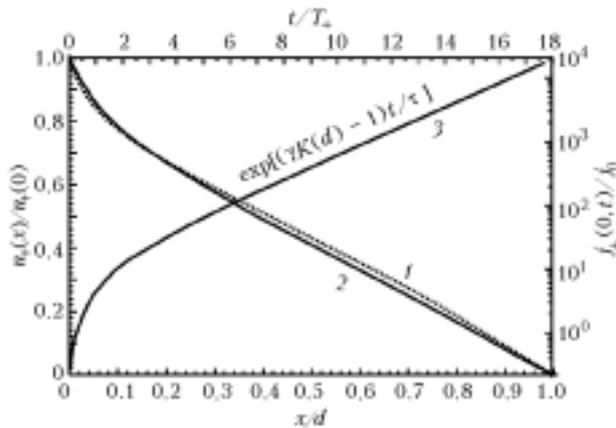
**Fig. 2.** Calculated ion density distribution over the length of the interelectrode gap at two moments in time:  $j_e(t_1)/j_0 = 10$  (1);  $j_e(t_2)/j_0 = 10^4$  (2), and the electron current density at the cathode as a function of time (3) at the following parameters: helium density of  $1 \cdot 10^{24} \text{ m}^{-3}$ ,  $d = 2 \text{ mm}$ ,  $U = 20 \text{ kV}$ ,  $\gamma = 0.6$ ,  $T_+ \approx 53 \text{ ns}$ ,  $\gamma K(d) - 1 = 0.3$ .
