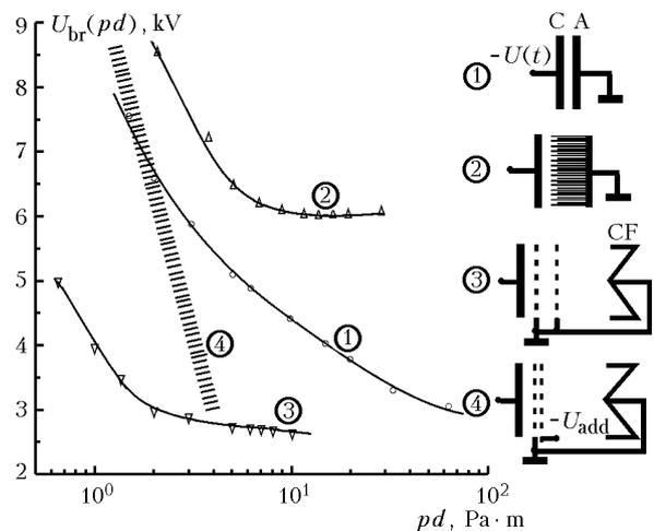
**Fig. 1.** Measured breakdown voltages for four versions of the discharge gap: versions 1 and 3 are borrowed from Ref. 1; C is the cathode, A is the anode, CF is the electron beam collector.
