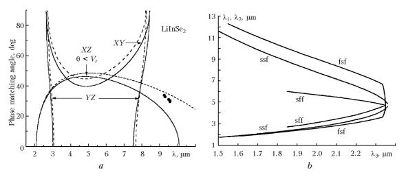
**Fig. 2.** Phase matching curves for SHG in the principal planes of the LiInSe<sub>2</sub> crystal according to data of this work (solid lines) and Ref. 16 (dashed lines); experimental data (dots) (*a*). The dependence of the wavelengths  $\lambda_1$  and  $\lambda_2$  of femtosecond pump pulses, for which sum frequency generation with pulse compression takes place in the plane *XY*, on the wavelength  $\lambda_3$  of the sum frequency radiation (*b*).
