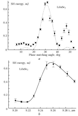
**Fig. 3.** Energy of the second harmonic of the 9R(22) line of the CO<sub>2</sub> laser at the room temperature versus angular detuning from the phase matching direction (the curve is an estimation result) (*a*) and the pump wavelength (the curve is approximation by least-squares method) (*b*).
