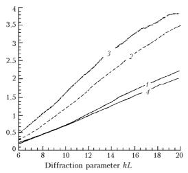
**Fig. 3.** The extinction efficiency factor of randomly oriented ice hexagonal cylinders (L/d = 6) calculated using the FDTD method (1), equivolume (2) and equisurface (3) spherical particles<sup>4</sup> and by means of the equivalent ensemble of spherical particles (4).
