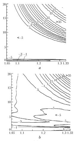
**Fig. 2.** Relative error  $\Delta$  (%) in calculating the extinction coefficients of the ensemble of randomly oriented oblate ( $\varepsilon = 2, a$ ) and elongated ( $\varepsilon = 0.5, b$ ) round cylinders by means of the equivalent ensemble of spherical particles as a function of the relative refractive index  $m_r$  and the maximum diffraction parameter  $\rho_{max}$ ;  $\varepsilon$  is the ratio of the base diameter to the length of the cylinder.
