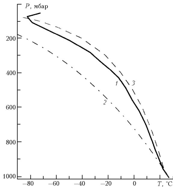
**Fig. 2.** *PT*-curves for the atmosphere above the ocean surface: measured in the equatorial zone (1), calculated for the ascending trial volume of dry air (2), calculated for the ascending trial volume of air with the relative humidity of 85% at the level of 10 m above the surface (3). Air temperature near the ocean surface is 27°C.
