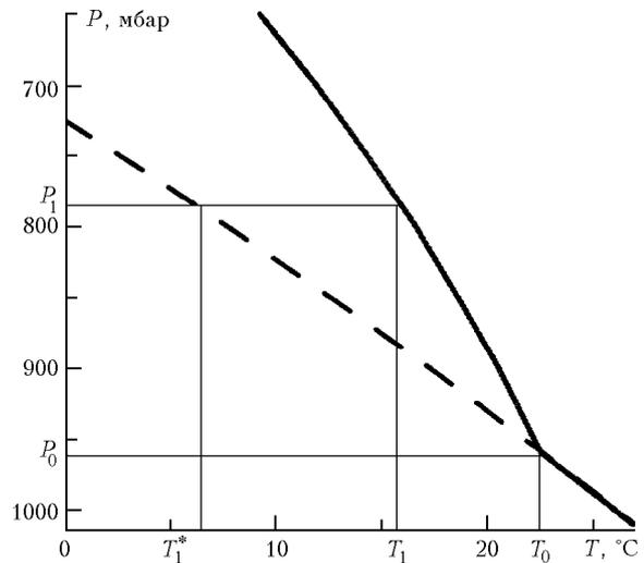
**Fig. 1.** Temperature conditions of trial air volume rising from the ocean surface; air temperature near surface is 27°C, relative humidity is 85%; dry adiabat (dashed line), adiabatic expansion of humid air (solid curve);  $P_0$  is the height (in units of pressure), at which water vapor begins to condense.
