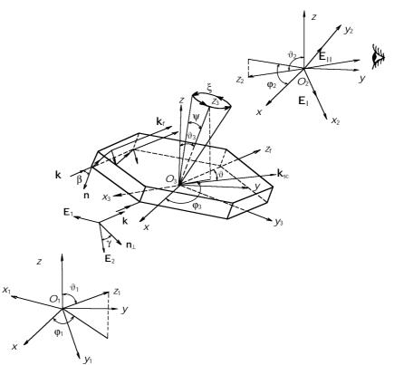
Fig. 1. The set of the coordinate systems for description of the light scattering into the forward hemisphere.
