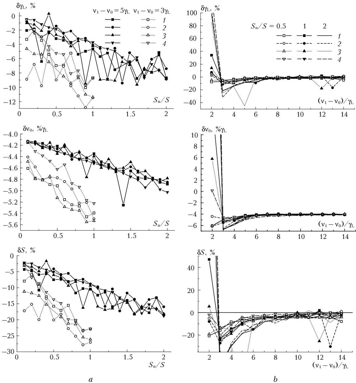
Fig. 7. Relative errors in parameters of the studied line retrieved from the fragment of the derivative of the spectrum vs. the intensity (a) and the separation (b) of the neighboring line.
