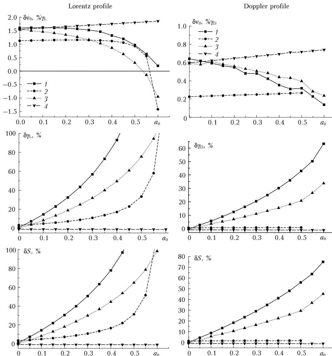
Fig. 2. Relative errors of line parameters retrieved from the spectral fragment vs. the background constant  $a_0$ .
