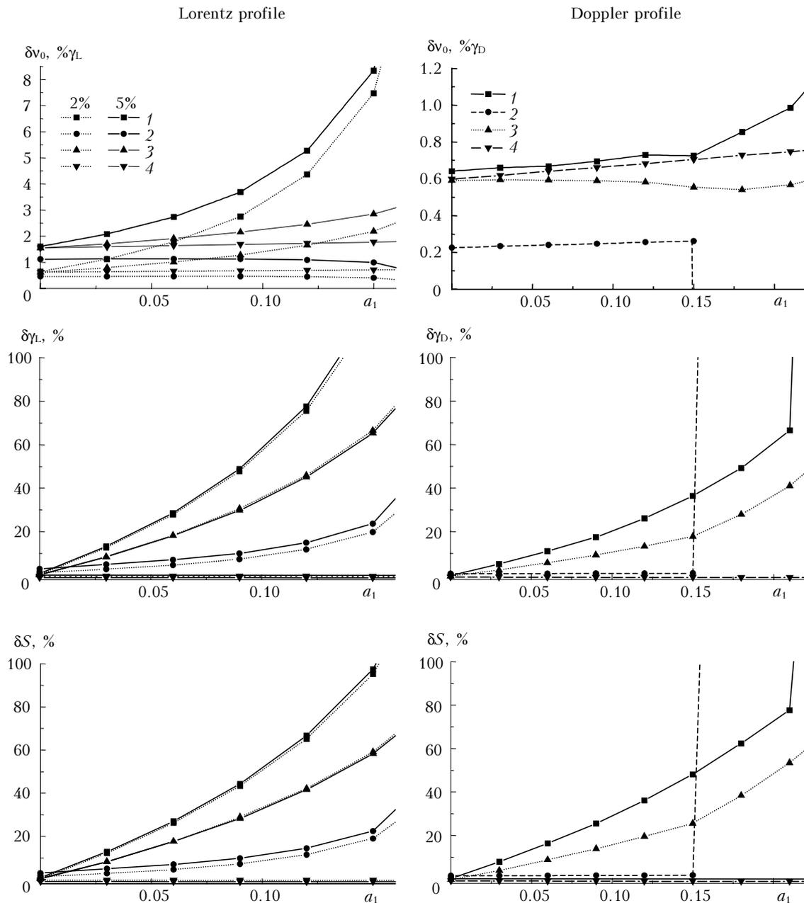
Fig. 3. Relative errors of line parameters retrieved from the spectral fragment vs. the background slope  $a_1$ .
