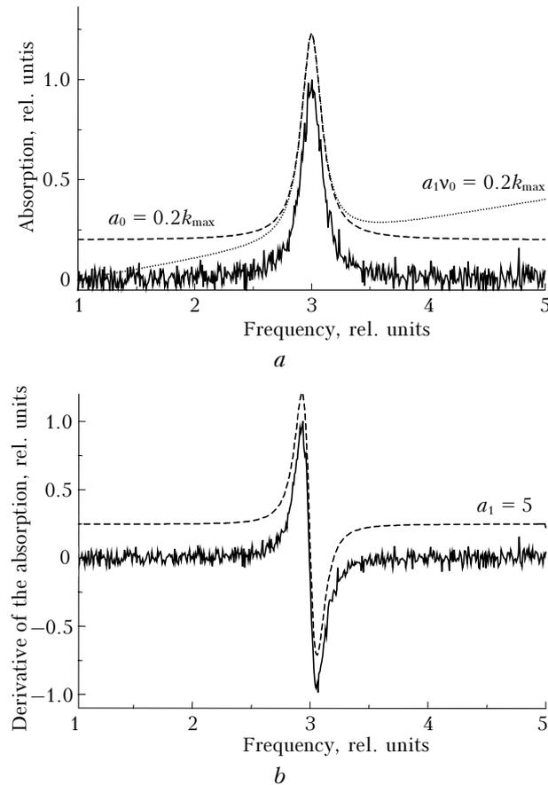
Fig. 1. Example of the model spectrum (*a*) and the spectrum derivative (*b*) with 5% random noise and linear background.
