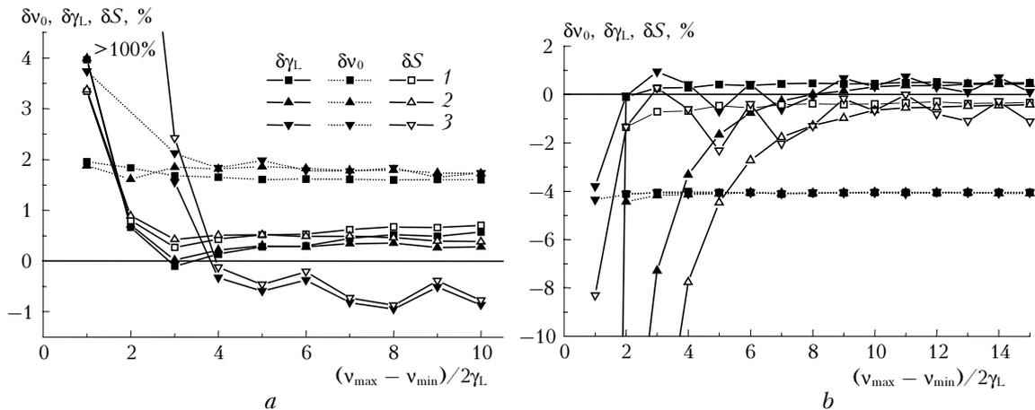
**Fig. 5.** Relative errors in parameters of the studied line retrieved from the fragment of the spectrum (*a*) and its derivative (*b*) vs. the width of the spectral fragment.
