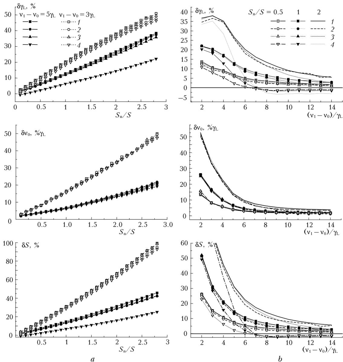
**Fig. 6.** Relative errors in parameters of the studied line retrieved from the fragment of the spectrum vs. the intensity (*a*) and the separation (*b*) of the neighboring line.
