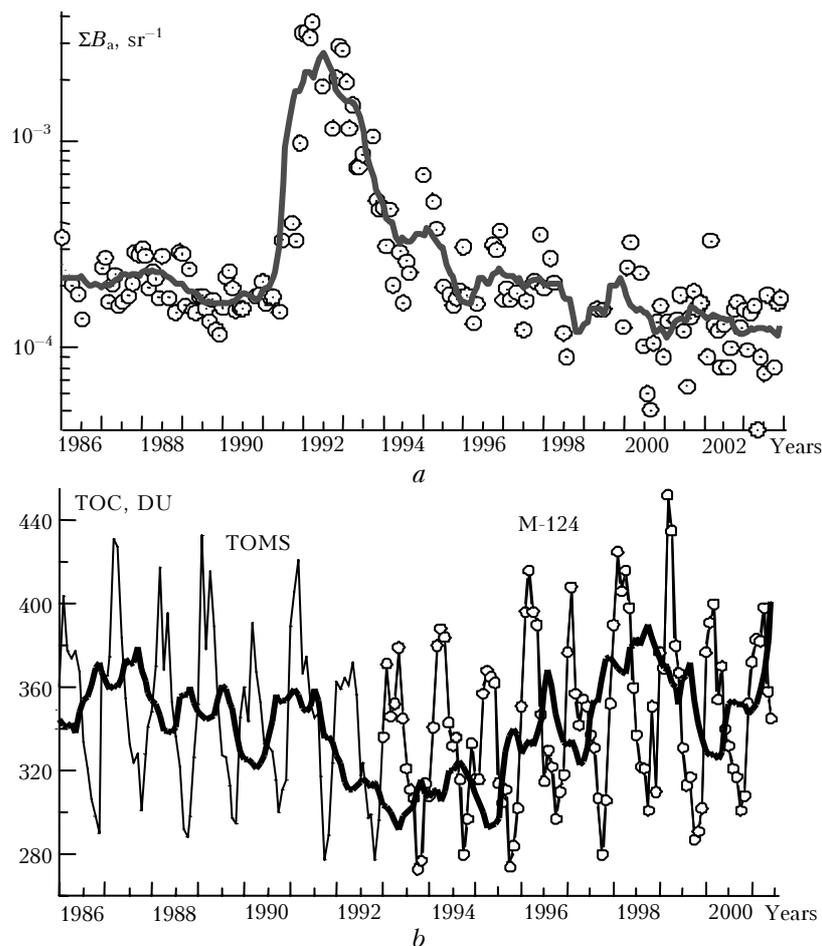
**Fig. 1.** Time variations of the integral aerosol backscattering coefficient in the layer of 15–30 km for the wavelength of 532 nm (*a*) and the total ozone content at mid-latitudes of the Northern hemisphere during the corresponding period (*b*). Time variations of the relevant parameters after smoothing by a moving average method with a window of 12 months are shown by heavy lines.
