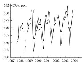
**Fig. 1.** Time behavior of the monthly mean  $CO_2$  concentration in the atmospheric layers of 0.5 to 2 (1) and 3 to 7-km heights (2), obtained from monthly airborne measurements from onboard the An-30 Optik-E flying laboratory over forests of Southwestern Siberia.
