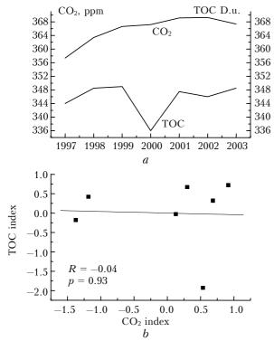
Fig. 5. Annual variations of the  $CO_2$  concentration and TOC (*a*) and the correlation between the TOC and  $CO_2$  indices at the height of 7 km (*b*).
