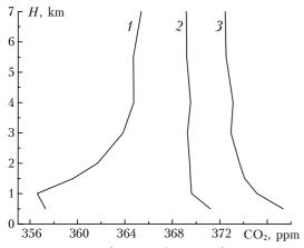
Fig. 2. Comparison of seasonal mean (summer, winter) and annual mean vertical profiles of  $CO_2$  obtained from the results of airborne measurements: summer (1), annual mean (2), winter (3).
