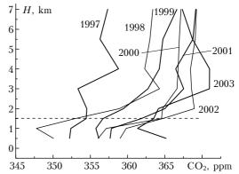
Fig. 3. Vertical  $CO_2$  profiles (the horizontal dashed line shows the level of 1.5 km).
