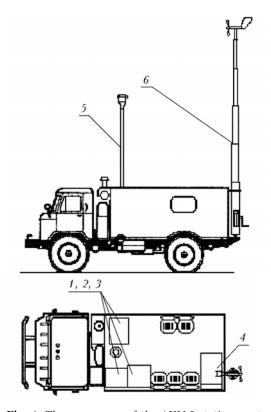
**Fig. 1.** The appearance of the AKV-2 station: posts with the measuring instrumentation (1, 2, and 3); power module (4); aerosol-gas intake (5); meteorological station based on the telescopic mast of KhZh4.115.025Sp type (6).
