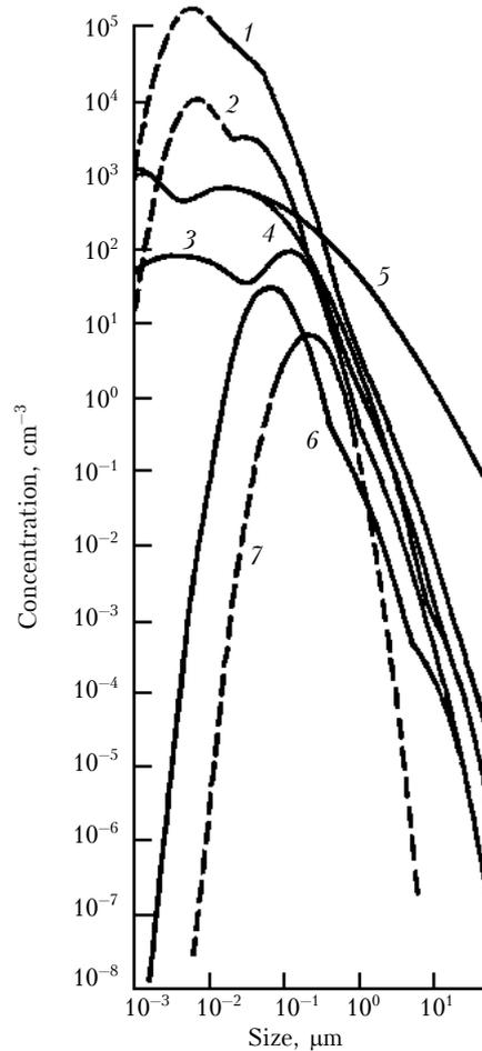
**Fig. 1.** The distribution of aerosol particles concentration over size<sup>13</sup>: urban (1); industrial (2); background (3); remote continental (4); dust storms in deserts (5); polar (6); stratospheric (7) aerosols.
