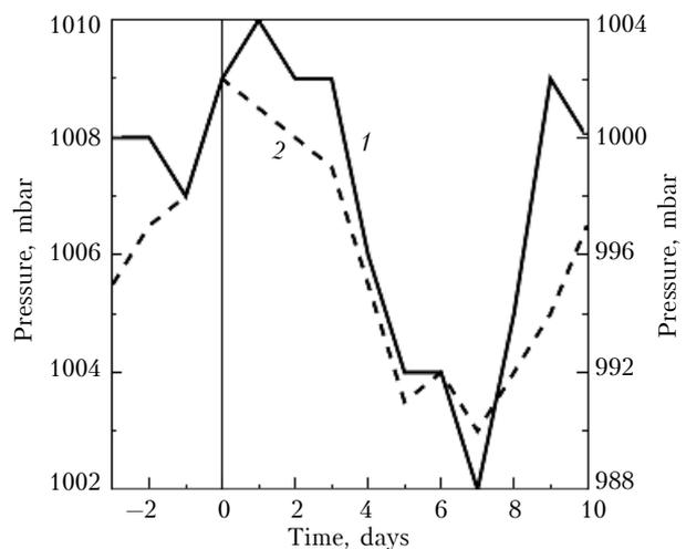
**Fig. 7.** Atmospheric pressure variation at the Earth’s surface after the SCR invasion in some regions of the Northern (1) and Southern (2) hemispheres obtained by the method of superposed epochs. Zero is the day corresponding to the moment of the SCR invasion. Scale on the left is the pressure in the Northern hemisphere.
