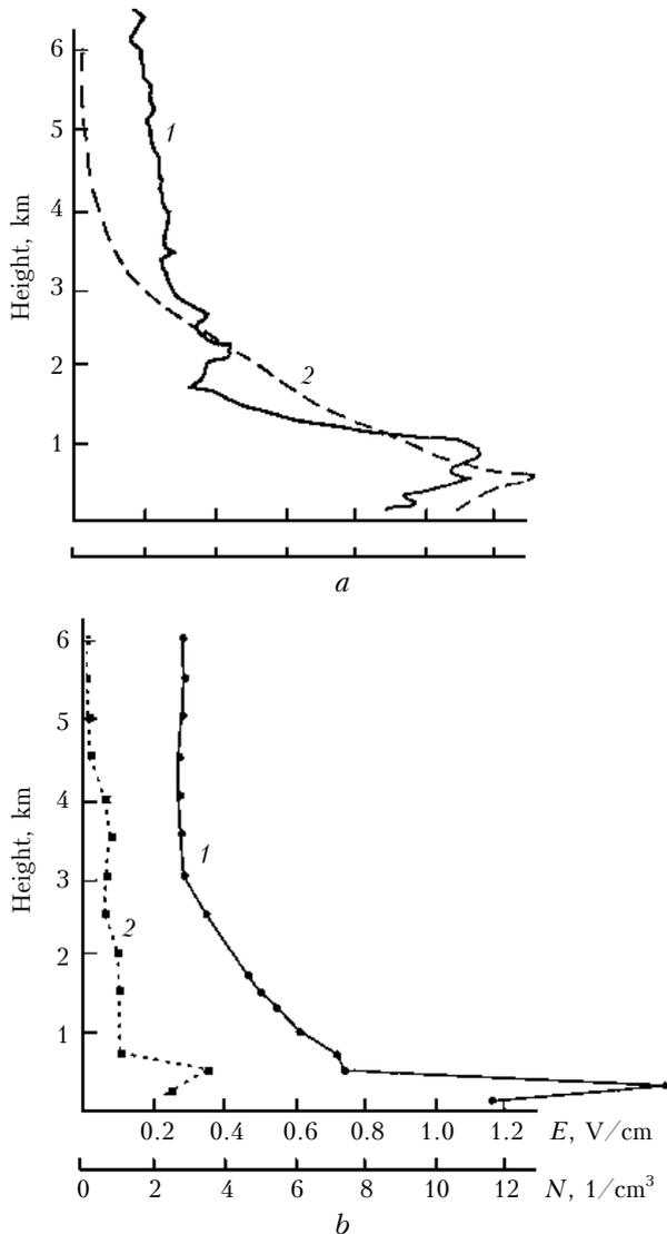
**Fig. 2.** Variations of height distribution of the condensation nuclei ( $N$ -curves 2) at the electric field variations ( $E$ -curves 1).<sup>15</sup>
