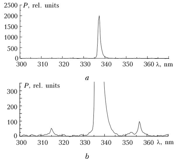
**Fig. 4.** Emission spectrum of nitrogen laser pumped with the generator with an inductive energy storage: the mixture is  $\text{N}_2/\text{NF}_3 = 75/3$  Torr,  $U_0 = 35$  kV,  $U_p = 25$  kV,  $C_p = 10$  nF, (a) attenuated by 250 times; (b) with the attenuation by 50 times.
