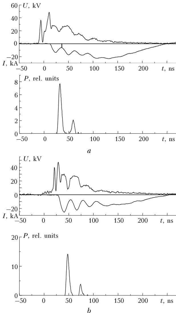
**Fig. 3.** Oscillograms of the voltage pulses at the discharge gap, discharge current, and laser pulse: the mixture is  $\text{N}_2/\text{NF}_3 = 75/3$  Torr;  $C_p = 10$  nF;  $C_0 = 70$  nF;  $C_1 = 2.45$  nF;  $U_p = 27$  kV;  $U_0 = 35$  kV; (a) is the laser with the capacitive energy storage; (b) is the laser with the inductive energy storage.
