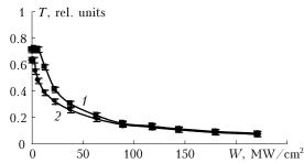
Fig. 5. Transmittance of the studied aluminum-based nonlinear media as a function of the excitation power density. Excitation at 532 nm, particle size: up to 600 nm (1), from 2600 nm (2).
