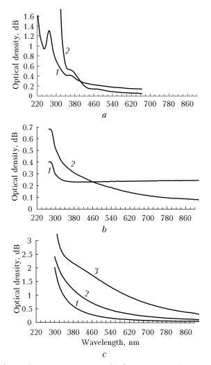
**Fig. 1.** Absorption spectra of dispersions with NPs: (*a*) platinum, particle size: up to 10 nm(1), up to 100 nm(2); (*b*) aluminum, particle size: up to 600 nm(1), from 2600 nm (2); (*c*) ATO, particles size: from 200 to 400 nm (1), from 200 to 400 nm (with micron-sized particles up to 2% of the mass) (2), from 400 to 1050 nm (with micron-sized particles up to 10% of the mass) (3).
