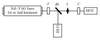
**Fig. 2.** Schematic of the experimental setup for investigation of the dependence of the medium transmittance on the power density of the exciting radiation: neutral-density filters F, beam-splitting plate BS, lens L, cell with the studied solution C, ED-100A pyroelectric detectors DET1, 2.
