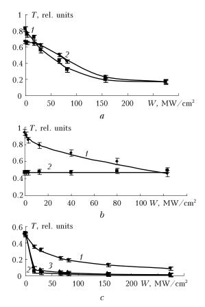
**Fig. 3.** Transmittance of the studied platinum-based nonlinear media as a function of the excitation power density: (*a*) excitation at 532 nm, NPs with the size up to 10 nm (1) and 100 nm (2); (*b*) excitation at 1064 nm, NPs with the size up to 10 nm (1) and 100 nm (2); (*c*) excitation at 532 nm, NPs with the size up to 10 nm (1), PC792 dye (2), and 1:1 mixture of the media 1 and 2 (3).
