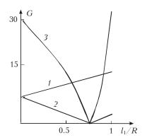
**Fig. 4.** Dependences of *G* coefficients of the interferometer sensitivity for the fixed values of f = 220 mm,  $l_1 = 200$  mm,  $l_2 = 160$  mm:  $G_1(1)$ ;  $G_2(2)$ ;  $G_3(3)$ .
