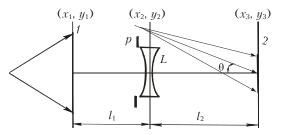
**Fig. 1.** Optical arrangement of the double-exposure recording of the quasi-Fourier hologram: 1 is the matte screen; 2 is the photographic plate; L is the negative lens; p is the aperture diaphragm.
