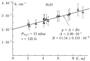
**Fig. 6.** The dependence of absorption coefficient of water vapor for Ti:Sa-laser FS-pulse ( $\tau = 120$  fs) on the pulse energy;  $dk/dE = (1.54 \pm 0.20) \times 10^{-8}$  cm<sup>-1</sup> · mJ<sup>-1</sup>.
