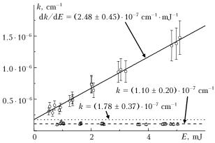
Fig. 4. Absorption coefficient of air for Ti:Sa-laser radiation depending on the laser pulse energy at  $\tau = 9$  ns ( $\Delta$ ) and  $\tau = 190$  fs ( $\circ$ ).
