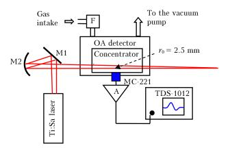
**Fig. 1.** Optical arrangement and block-diagram of the OA spectrometer: M1 is a plane mirror, M2 is a spherical mirror with F = 86.5 cm; F is an aerosol filter; A is a wide-band amplifier with the gain coefficient of 1000; MC-221 is the half-inch microphone.
