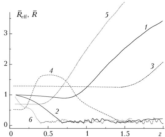
**Fig. 5.** Effective (1, 3, 5) and geometric radii (2, 4) of collimated beams of Gaussian (1, 2), ring (3, 4) with  $p = 0.5$ , and super-Gaussian ( $q = 8$ ) cross section (5, 6) along the path at  $\eta = 5$ .
