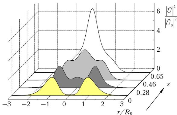
Fig. 6. The cross section of relative intensity of a collimated ring beam ( $p = 0.5$ ) along the path at  $\eta = 5$ .
