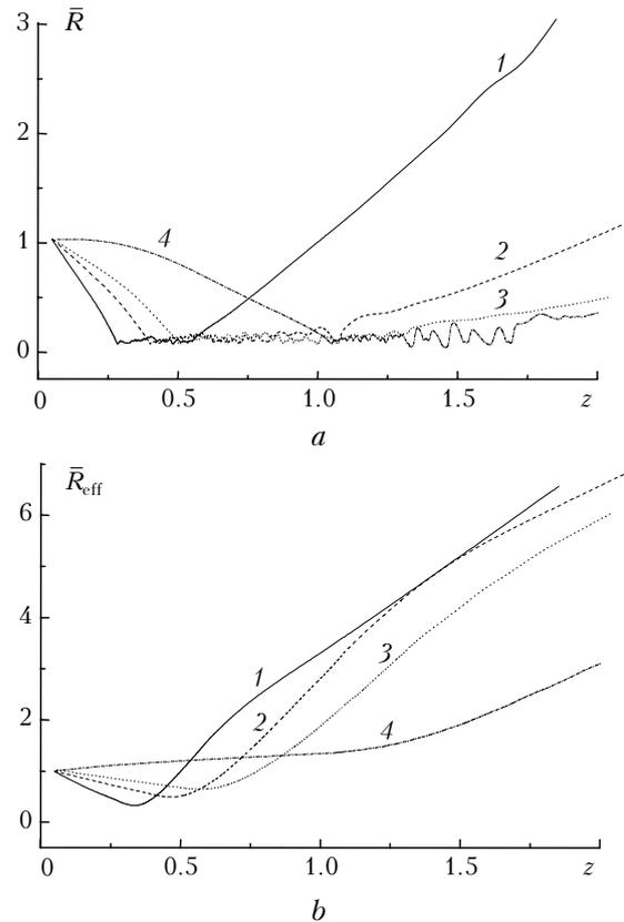
**Fig. 1.** The dependence of normalized values of geometrical  $\bar{R} = R(z) / R_0$  (a) and the effective  $\bar{R}_{\text{eff}} = R_{\text{eff}}(z) / R_0$  (b) radii of a femtosecond pulse with  $\eta = 5$  and  $F = 0.5$  (1); 1 (2); 2 (3), and  $-2$  (4) on the distance along the propagation path.
