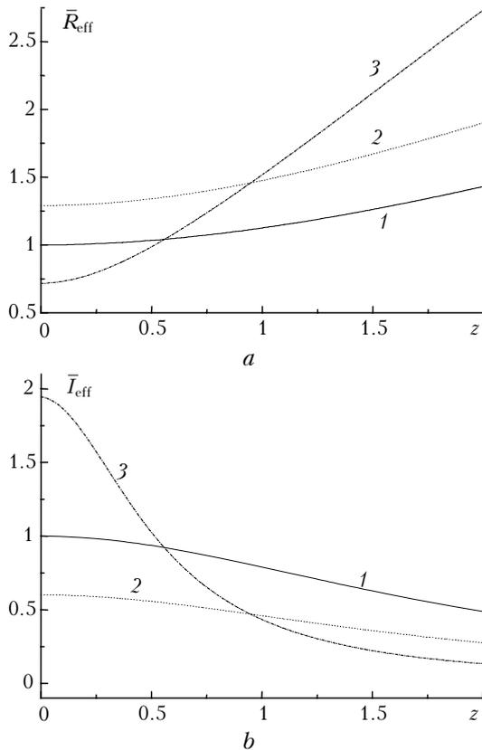
**Fig. 4.** The dependence of the effective radius (a) and mean intensity (b) of collimated beams of Gaussian (1), ring (2) with  $p = 0.5$ , and super-Gaussian ( $q = 8$ ) cross section (3) on the space variable.
