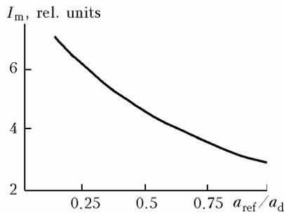
**Fig. 1.** Maximum intensity  $I_m$  in the cross section of a focused laser beam as a function of the size of a reference source. Abscissa shows the ratio of the size of the reference source to the size of the diffraction limited beam  $a_d$  in vacuum. The distance is  $x = ka^2 = 0.25$ . Under conditions of thermal blooming without correction  $I_m = 1.1$ .
