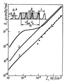
Fig. 1. Heart number of 9P(30) CO<sub>2</sub> laser photons absorbed by O<sub>3</sub> molecules versus laser intensity at 3 torr and 300 K. Points for experimental results from Ref 4.
