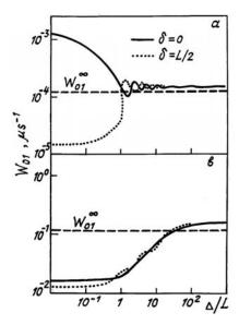
Fig 3. Vibrational transition excitation probability approximated by Elsasser band versus continuous radiation width for fixed total intensity: a) – for  $I = 10 \text{ W/cm}^2$ , b) – for  $I = 10 \text{ kW/cm}^2$ . Band parameters are the same as in Fig. 2.
