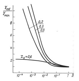
FIG. 2.  $\gamma_{col}/\gamma_{min}$  vs  $\beta$  for different normalized values of thickness  $Z_s$  of the nonlinear layer.
