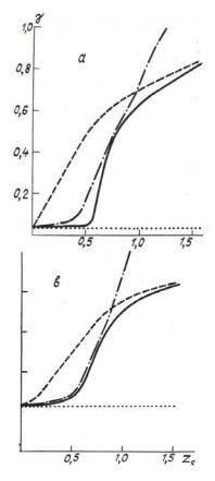
FIG. 1. The angular divergence  $\gamma$  versus the normalized values of the . thickness  $z_s$  of the factor of the nonlinear layer with  $\beta = 0.001$  (a) and  $\beta = 0.05$  (b). The solid line corresponds to the optimally focused beam, the dashed line corresponds to a collimated beam, the dot-dashed line was calculated using the algorithm, and the dotted line shows the diffraction limit.
