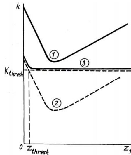
FIG. 3. Explanation of the tracing-paper experiment: 1 – the contrast for observation of luminous objects; 2 – external illumination of reflecting objects; 3 – the apparent dependence  $k = k(z_1)$ .
