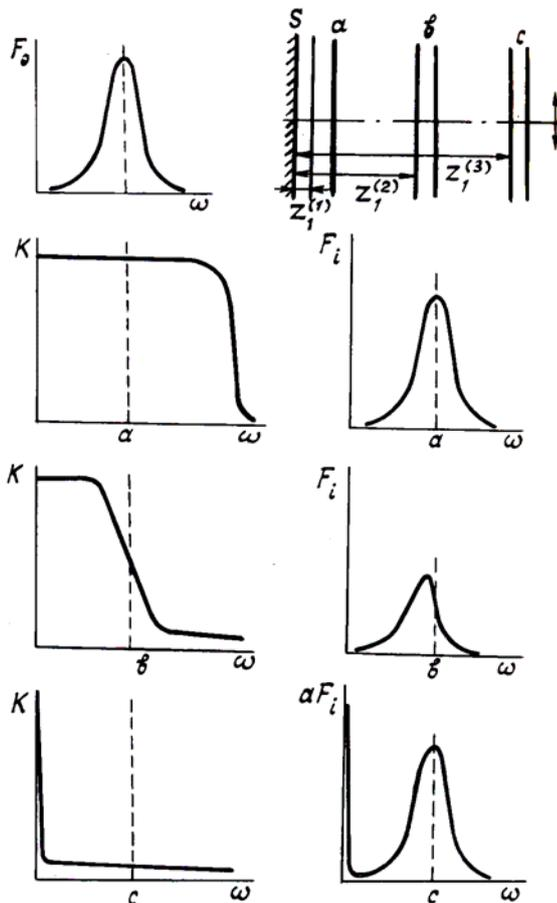
FIG. 4. Explanation of the  $t$ -effect.  $F_0(\omega)$  is the spectrum of the object;  $K(\omega)$  is the frequency-contrast characteristic; and,  $F_i(\omega)$  is the spectrum of the image.
