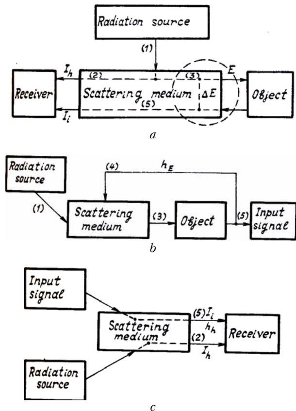
FIG. 2. Block diagram of the process of image transfer through a scattering medium.
