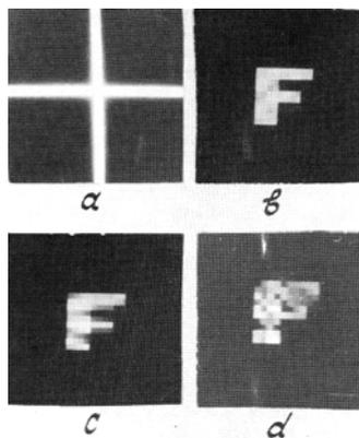
FIG. 1. a – the spatial frequency band in which information about the spectrum or its component is given; b – the image reconstructed from the spectrum given in the region of the "cross"; c – the image reconstructed only from the phase of the spectrum given in the region of the "cross"; d – the initial estimate of the image reconstructed from the modulus of the spectrum, extrapolated from the region of the "cross" to the entire frequency plane.
