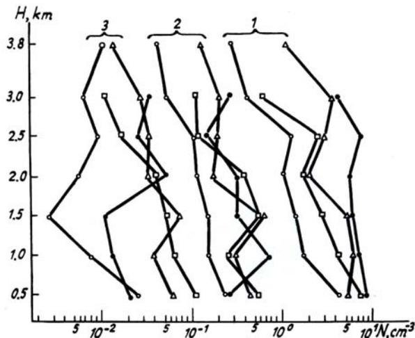
FIG. 2. The vertical distribution of the aerosol above Kazakhstan for the fractions  $d = 0.4-0.5 \mu\text{m}$  (1),  $d = 0.8-0.9 \mu\text{m}$  (2), and  $d = 4-7 \mu\text{m}$  (3) with different humidity (see FIG. 1 for an explanation of the labeling).
