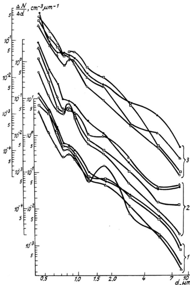
FIG. 3. The distribution of aerosol particles over the spectrum above Western Siberia at altitudes of 600 m (1), 2500 m (2), and 4000 m (3) for different values of the humidity (the labeling is explained in Fig. 1).
