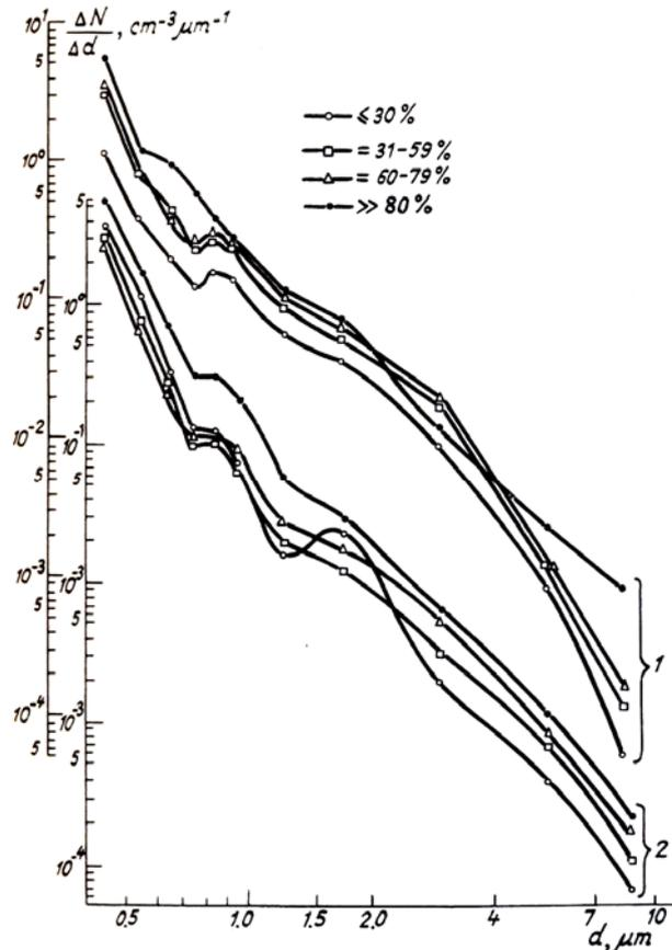
FIG. 1. The aerosol particle distribution according to the spectrum above Kazakhstan (1) and Western Siberia (2) with different humidity.
