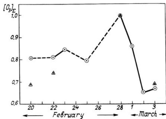
FIG. 2. The relative integrated ozone concentration in the layer (lidar measurements denoted by triangles) and in the entire atmosphere (Dobson meter marked by circles) as a function of time.
