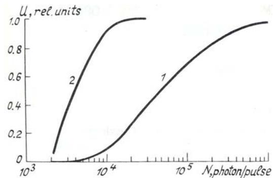
FIG. 3. The average energy of a packet of pulses (1) and the average amplitude of a packet of pulses (2) versus the intensity of pulsed illumination.
