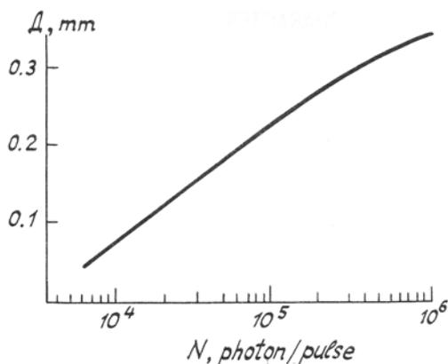
FIG. 2. The diameter read" versus the intensity of pulsed illumination.
