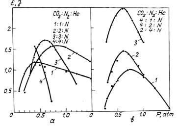
Fig. 3. The optimal dependences of the radiation energy on the content of CO<sub>2</sub>,  $N_2(a)$ , and  $N_2(b)$  and the total working pressure of the mixture with  $U_0 = 30$  kV.
