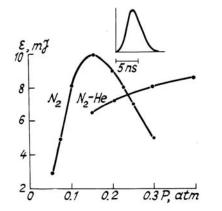
Fig. 4. The radiation energy as a function of the  $N_2$  and He content. The inset shows the radiation pulse of a  $N_2$  laser.
