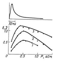
Fig. 1. The energy of radiation for the gas mixture  $CO_2:N_2:He = 1:1:N$  as a function of the helium content and the magnitude of the charging voltage: 20 kV (1), 25 kV (2), and 30 kV (3). The graph at the top shows the radiation pulse in a mixture with no helium  $CO_2:N_2 = 4:1$ .
