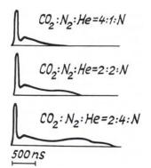
Fig. 2. Typical oscillograms of radiation for the gas mixtures  $CO_2:N_2:He$  with P = 0.6-1 atm.
