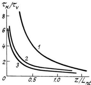
FIG. 2. Degradation of the temporal coherence of a laser beam along the propagation path with  $L = 10L_{nl}$  and  $\sigma_v/\nu_0 = 0.1$  (1), 0.3 (2), and 0.5 (3).
