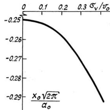
FIG. 1. The position of the energy center of the beam as a function of the standard deviation of the wind velocity fluctuations at a distance  $z = 0.5L_{n1}$ .
