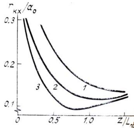
FIG. 3. The transformation of the coherence radius of the beam  $r_{cx}(z)$  along a propagation path with  $L_d = 10L_{nl}$  and  $\sigma_v/\nu_0 = 0.1$  (1), 0.3 (2), and 0.5 (3).
